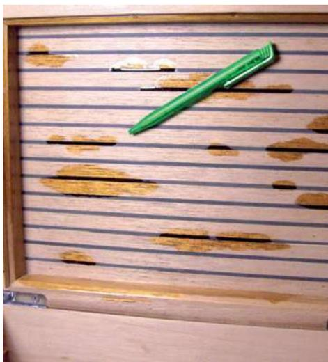
Left and right: An example of extreme "resin bleed" resulting from the use of too much Spanish cedar wood in a humidor
